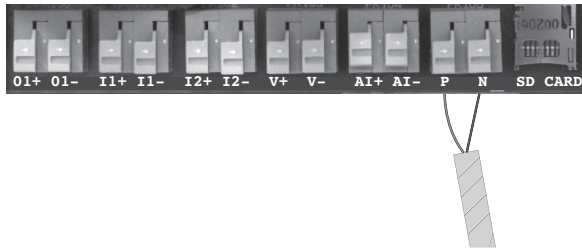
Figure 19 - Example RS-485 Connection
