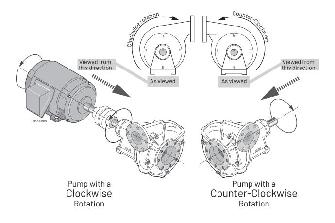
Pump Rotation is determined as clockwise or counter-clockwise by viewing liquid end of pump from the **back** or **shaft side**, and **NOT** from looking into the impeller eye or front of volute.
