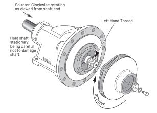
• Hold shaft stationary and remove impeller by turning in the direction shown for either clockwise or counter-clockwise pump rotation.
