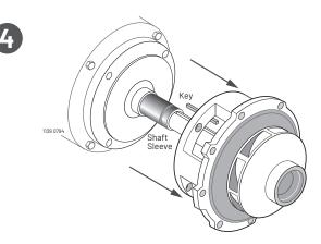
• If a seal retaining ring is part of the assembly, it will need to be replaced.
