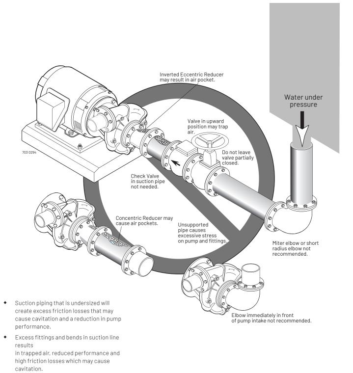
If a check valve is required for back flow prevention, locate on the discharge side of pump.
