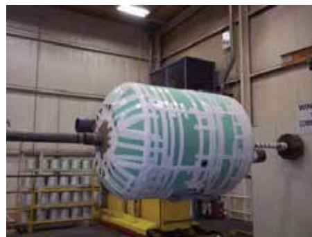
Insulated Vessel at Start of Winding
